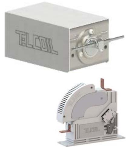
SI contactors poles terminals can be configured in 8 different shapes, allowing vertical plane („wall“) or horizontal plane („floor“) fixing without changing the pole orientation and its dynamic behaviour, i.e. without any setting or hardware difference in the poles. The terminal kits vary by current / shape and run inside container slots.
